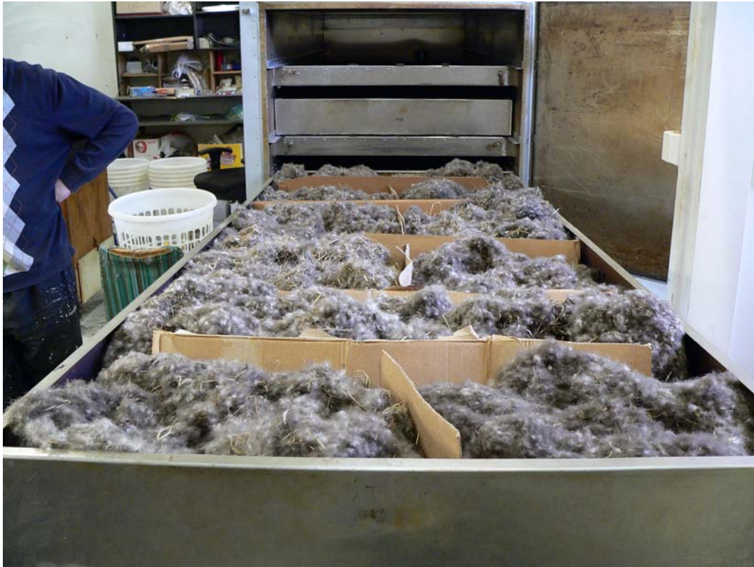
Figure 2. Special made oven designed to dry and sterilize eider down before cleaning. Photo: T. H. Carlsen.
