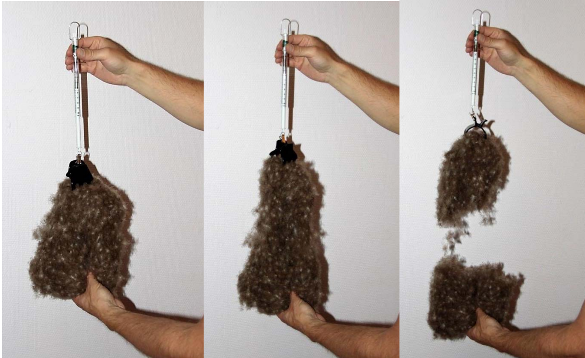
Figure 5. To measure the maximum cohesion of the sticky eider down, the sample was pulled downward away from the spring scale and the maximum force (expressed in g and converted to N) was measured the moment just before the down sample was teared apart. Photo: Liv Jorunn Hind.
